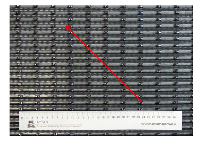
Figure 1: Maydel - Vynagrip - Industrial Matting Arrow indicates direction of testing
